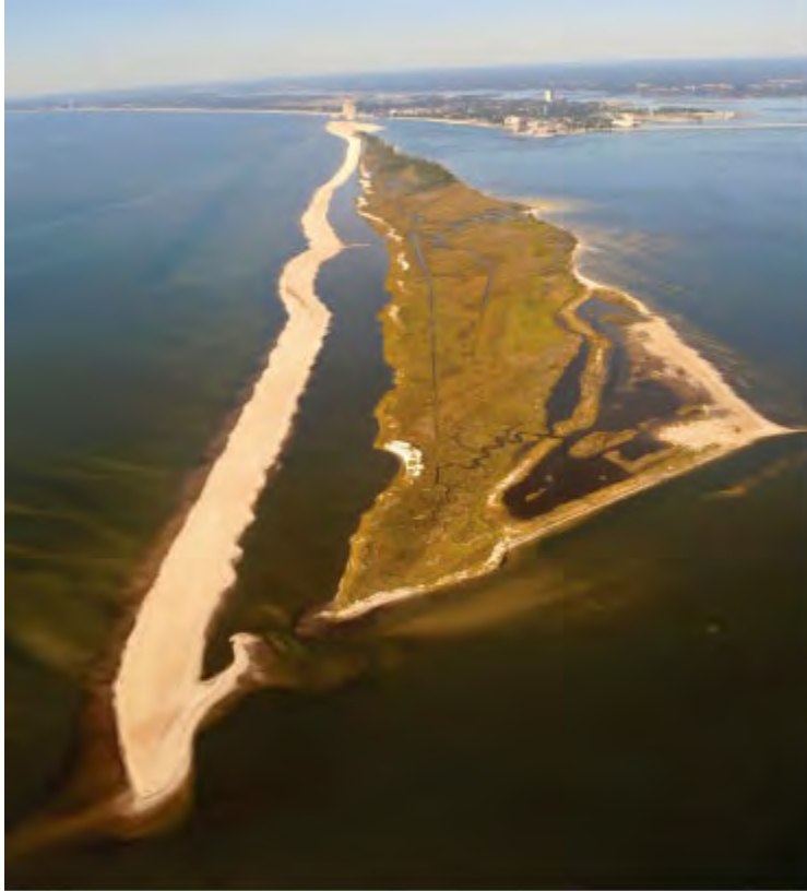
Figure B-3. Restored southern shoreline of Deer Island including lagoon created as a future beneficial use site. From Smith et al. (2015).
