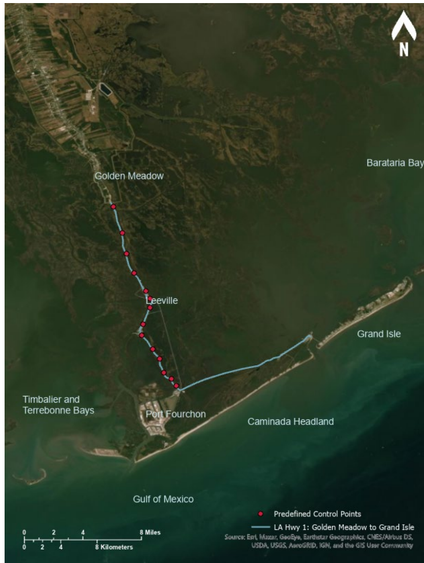
Figure 18. Data extraction points were located arbitrarily along the unelevated portion of LA 1 from Golden Meadow to Grand Isle.
