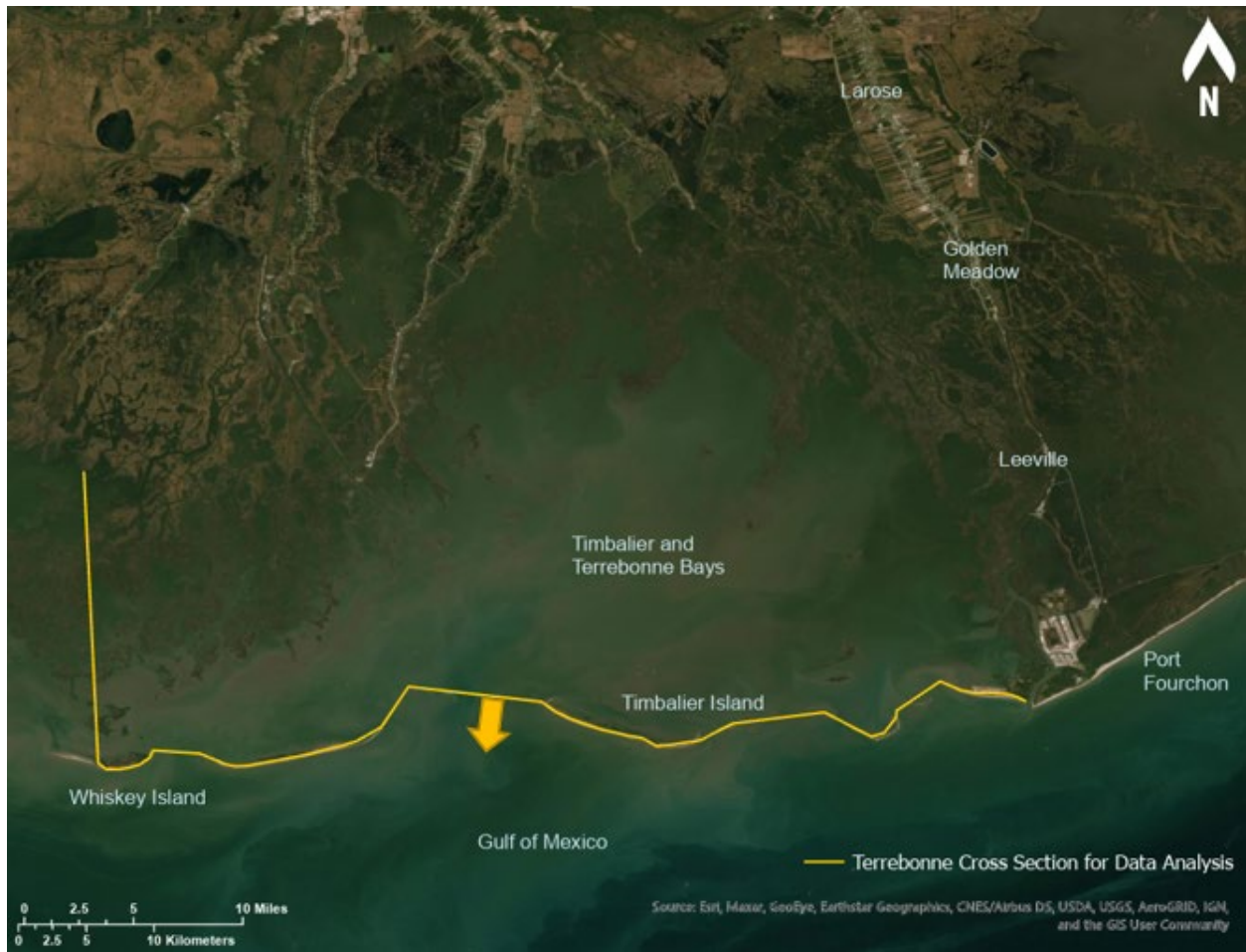
Figure 37. Cross-section along which model output were extracted for quantifying water and sediment fluxes along the barrier islands and tidal inlets of the Terrebonne Basin. Fluxes in southern (offshore) direction are positive as indicated by the yellow arrow
