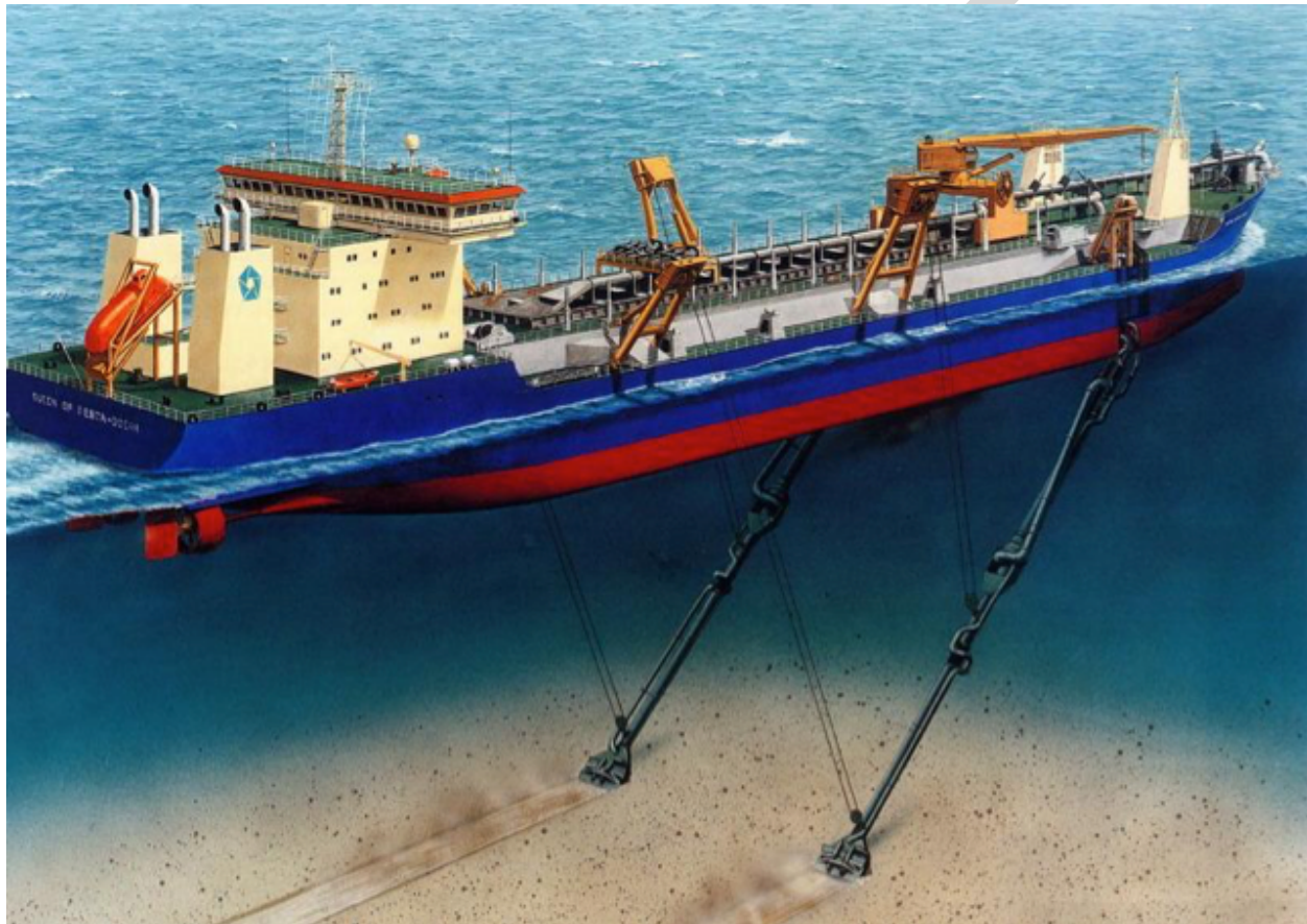
Figure 9. Trailing suction hopper dredge. A 7,000 yd 3 self-propelled TSHD. The trailing suction arms can be seen to the port and starboard sides of the vessel attached to boom cranes on the deck (Retrieved from: http://www.theartofdredging.com/stpmfordummies.htm ).
