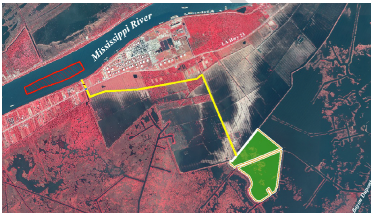
Figure 12. Bayou Dupont Restoration Area. Elements of project BA-39 illustrated above: borrow area (red), sediment pipeline (yellow), and marsh creation area (green). (Source: Thomas, 2007)
