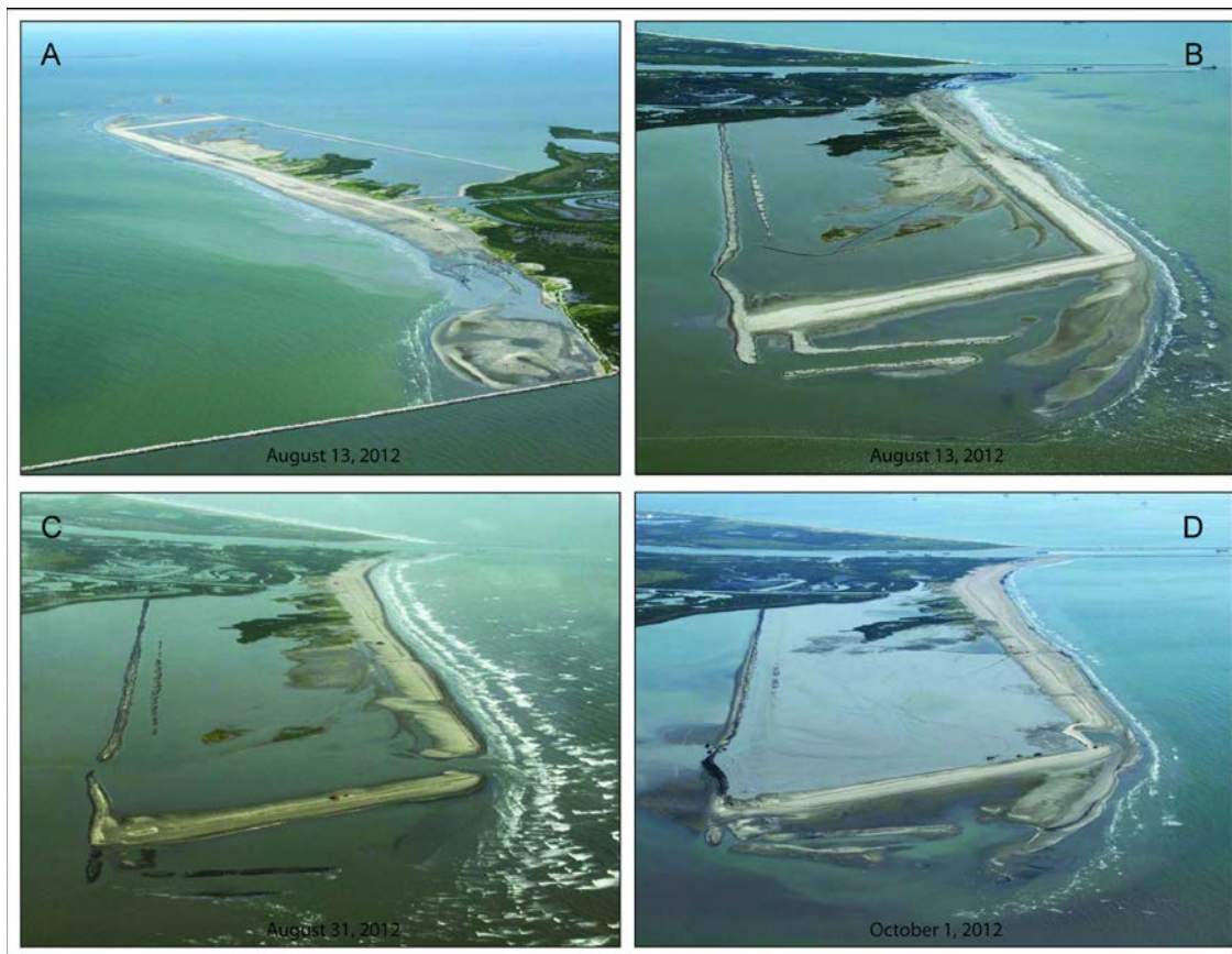
Figure 8: CPRA Restoration Project TE-52 performed on West Belle Pass Barrier, four photos show the containment dike and sediment renourishment progress. A) View from the east of project under construction on August 13, 2012. The west Belle Pass jetty is in the foreground. B) View from the west of project under Construction on August 13, 2012. with a recently formed recurved spit. C) View toward the east on August 31, 2012, after Hurricane Isaac passed directly over the barrier and created a breach in the containment dike and washover deposition of 104 yds 3 of sand. D) View from the west of project on October 1, 2012 after sheetpile closure of the containment dike breach. (Photographs from Weeks Marine & Aerophoto; Parker et al., 2012).
