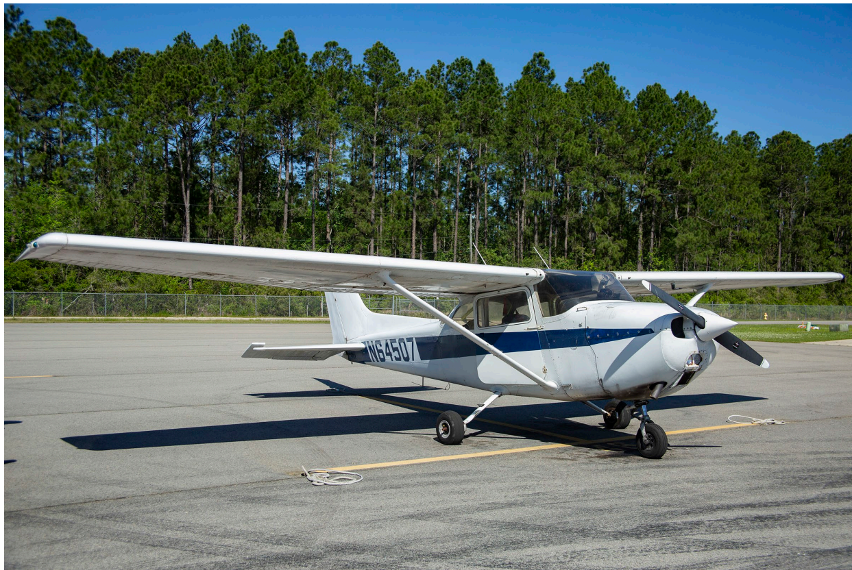
Figure 2. Photo of the aircraft used for the 2023 image acquisition. The aircraft was a Cessna 172M with extended fuel tanks.
