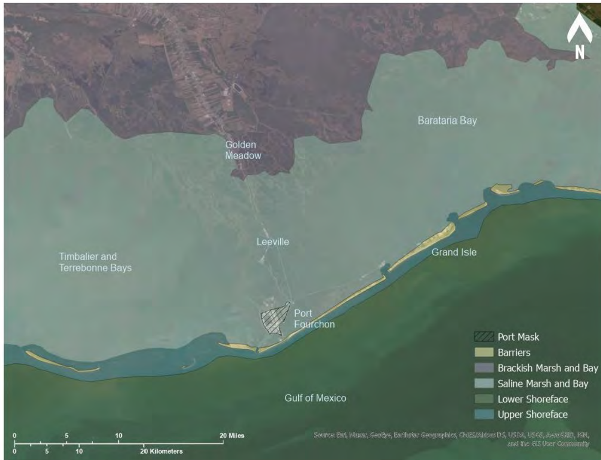
Figure A-14. Map with spatial delineation of sediment layers. See Table A-3 and Table A-4 for sediment layer classification by grain size. From north to south: brackish wetland (purple), saline wetland (teal), barrier (yellow), upper shoreface (blue), and lower shoreface (green). Note. Reprinted from previous study by The Water Institute of the Gulf (2022).
