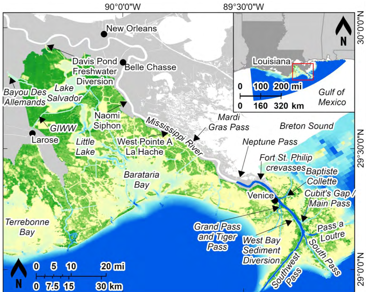
Figure A-13. Topobathymetric map of the model domain, showing all features that represent or are related to boundary conditions.
