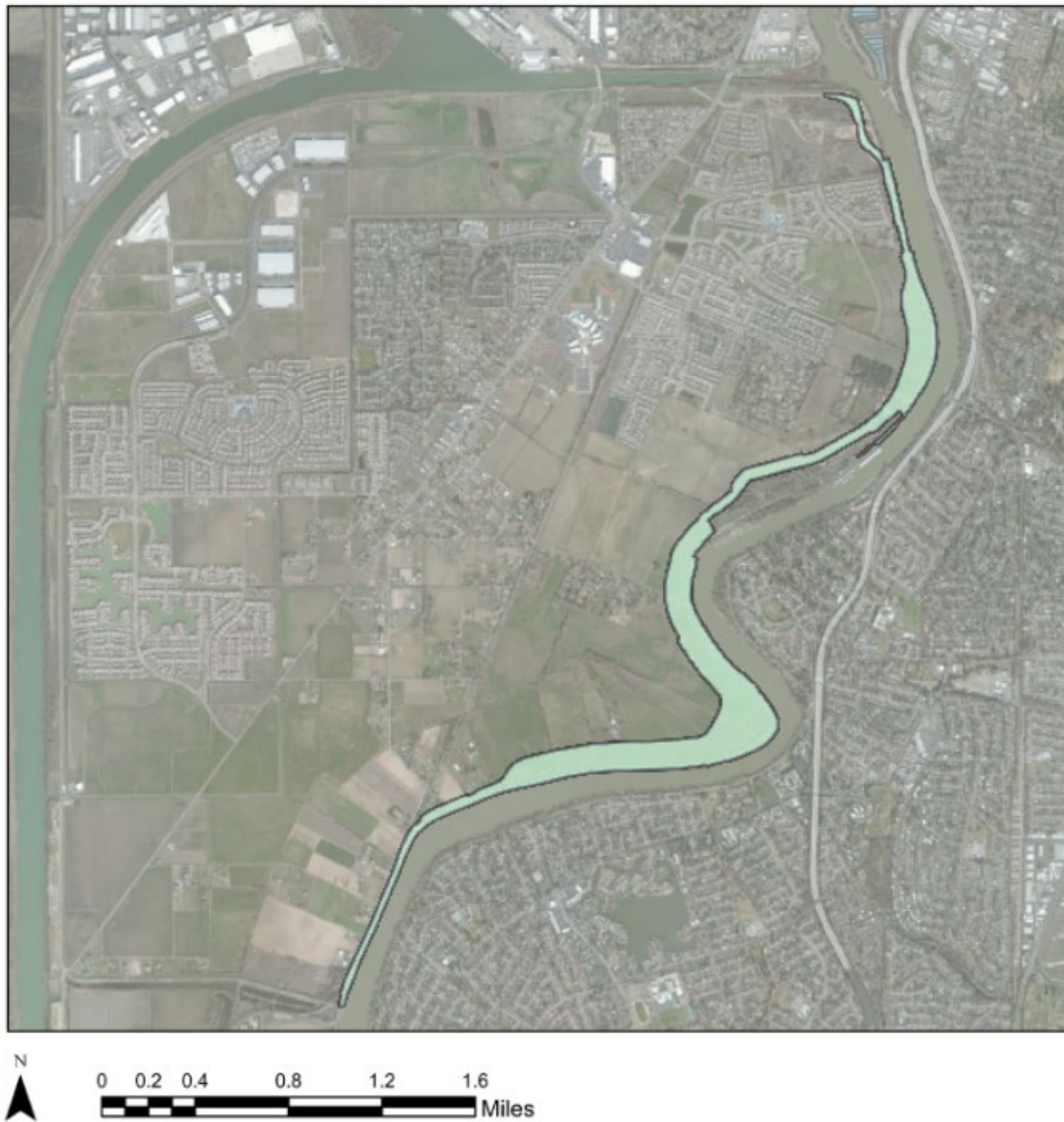
Figure 6-4. Location of proposed setback levee along Sacramento River, light green area indicates the 60 acres of river floodplain to be restored: A component of Alternative 5.
