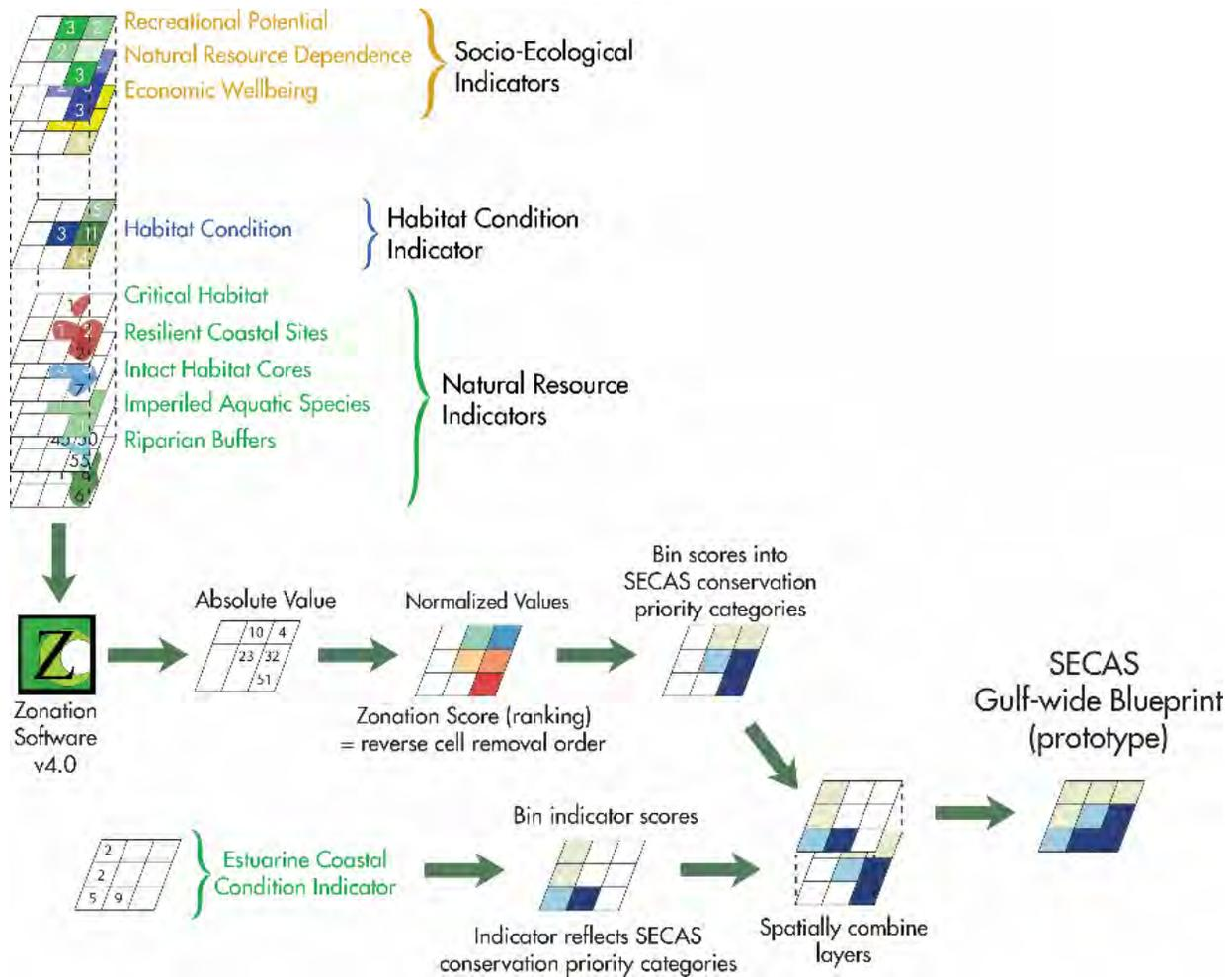
**Figure 4. Simple schematic of prioritization analysis using Zonation software.**
