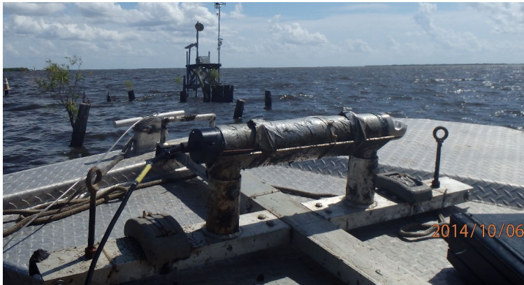
Figure 15. Photograph of Nortek Sidelooking Aquadopp current meter on sled mount resting on the vessel deck
