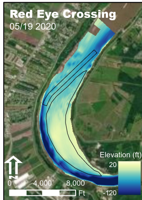
Figure 29. Bathymetric map of Red Eye crossing showing the point bar and thalweg. Black outlines delineate the crossing channel and the bar area.
