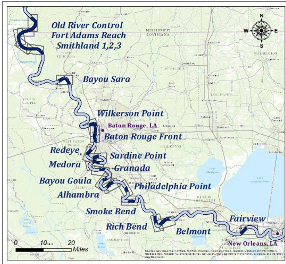
Figure 4. Mississippi River Crossings dredging reach. Shallow draft Crossings (maintained to -9 ft LWRP) extend from Old River Control to Wilkerson Point. Deep draft Crossings (maintained to -50 ft LWRP) extend from Baton Rouge Front to Fairview. Ten out of the 12 deep draft Crossings require maintenance on an annual basis, with Rich Bend and Fairview requiring maintenance on a less than annual basis (USACE, 2018b). Image sourced from (USACE, n.d.-b, accessed March 15, 2021).
