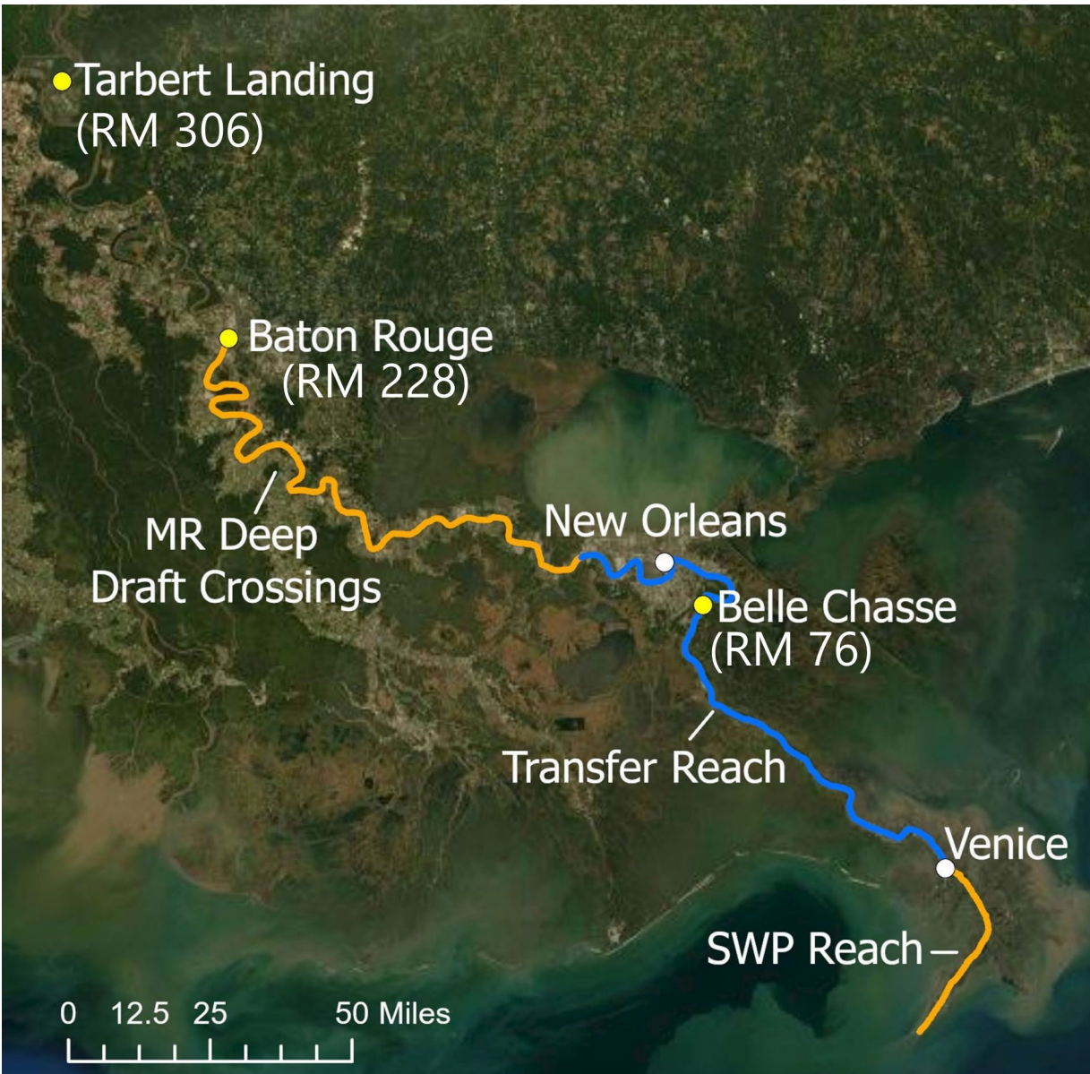
Figure 1. Map of study area showing the Mississippi River (MR) Deep Draft Crossings and the SWP reaches (orange lines), both of which require regular dredging to maintain authorized navigation depths. The Transfer Reach (blue line)—in which navigable depths occur without dredging—links the two dredged reaches. The gauge data used in this report are from Tarbert Landing (RM 306), Baton Rouge (RM 228), and Belle Chasse (RM 76), all shown as yellow circles.
