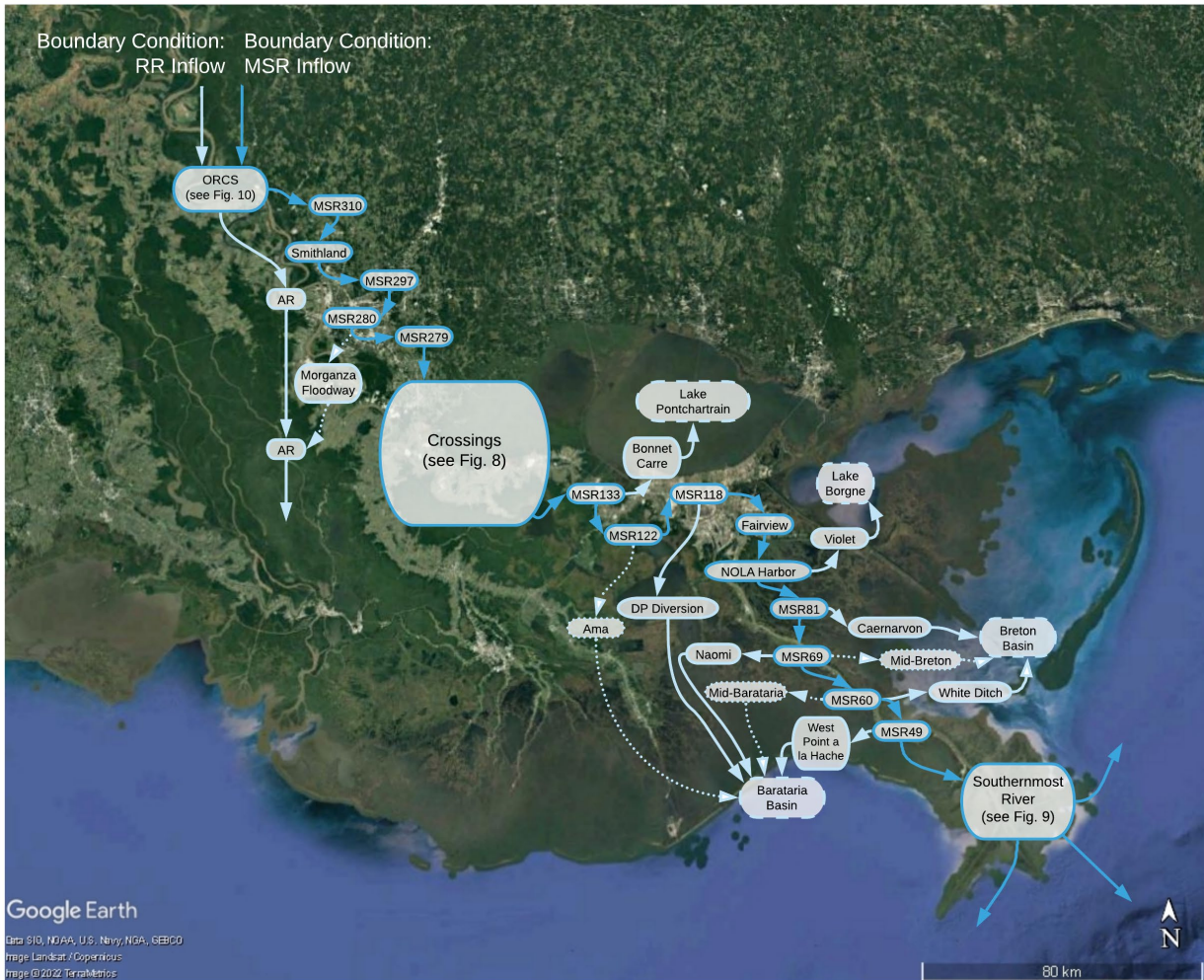
Figure 7. Draft stocks and flows that comprise the design of the environmental prediction module, which includes portions of the Mississippi River (MSR), Red River (RR), and Atchafalaya River (AR). Details of the Old River Control (ORCS) section of the LMR is shown in Figure 10; the Crossings section is shown in Figure 8; and the southernmost LMR section is shown in Figure 9. Dark blue borders indicate the main stem of the MSR model and light blue borders indicate outflows. Background imagery courtesy of Google Earth® and flow elements added with LucidChart®.
